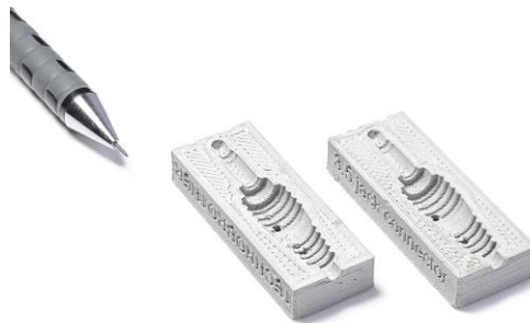
Fig. 1: Sintered mould cavity printed with CMG Tech-X H13 filament.
